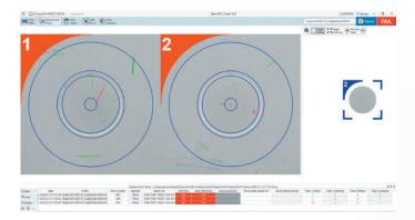
Thanks to its wide field of view camera, the Dscope MT allows to scan both ferrules of Duplex connectors in one shot whether it is LC Duplex or Very Small Form Factor connectors (CS, SN, MDC,...).
